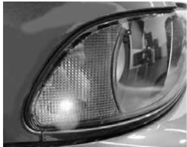
US version side marker reflector with wave guide illumination.
