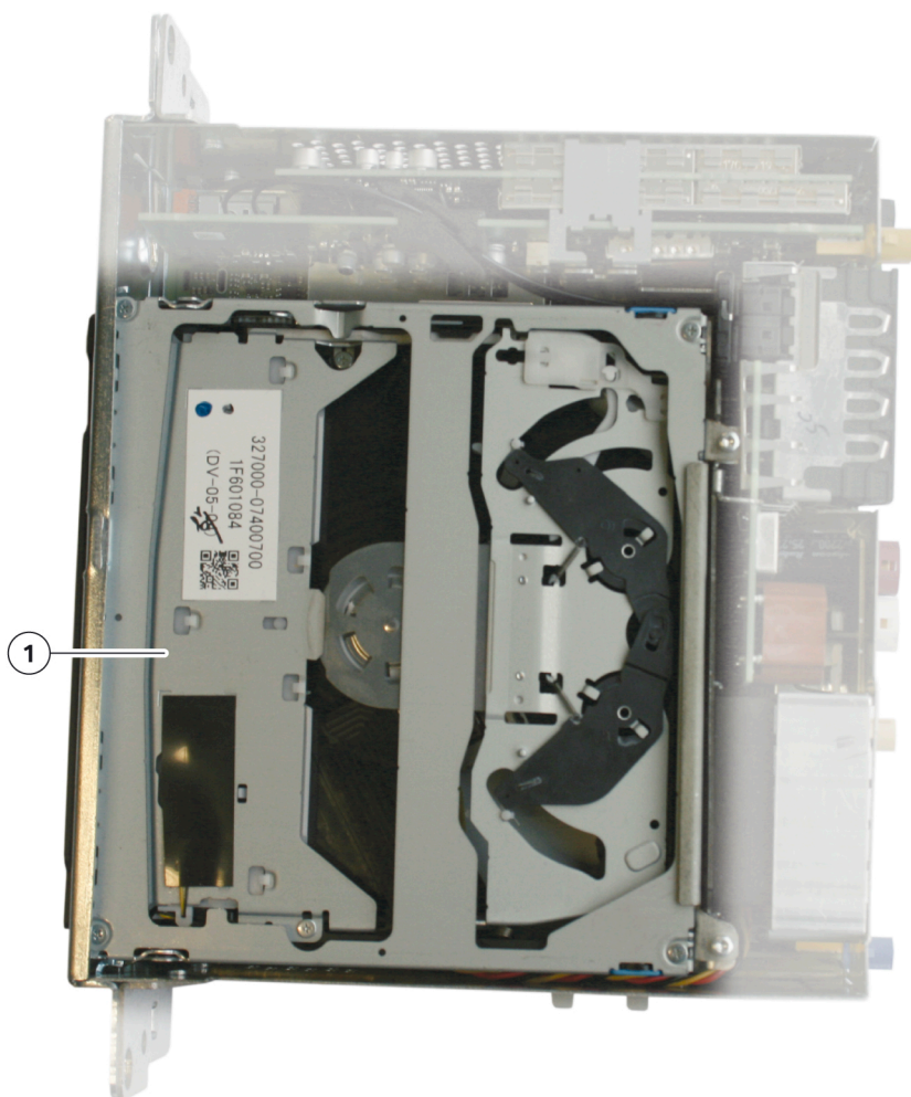
CD-ROM drive installed in a CIC Basic
