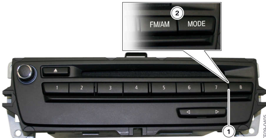
CIC Basic (front view) in the E9x and E8x series
