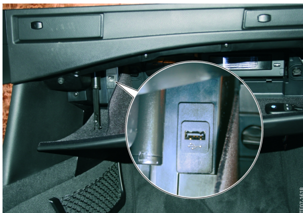
USB import interface in the glove compartment for uploading navigation data
