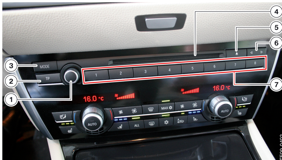
IHKA/audio control panel in the F07
