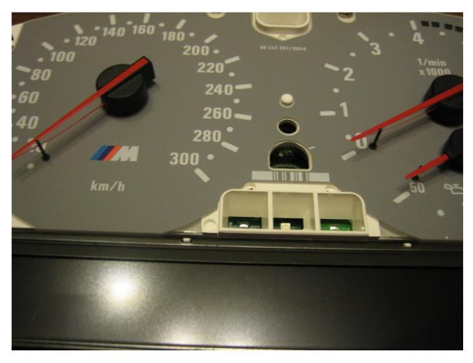
The hands of the fuel and temperature gauges require more attention being the pivots don't have a stopping point. It is for this reason that following the procedure precisely and referencing the photos is key. [Editors note- you can add a small indelible mark to try and get these parts aligned on reassembly.]
