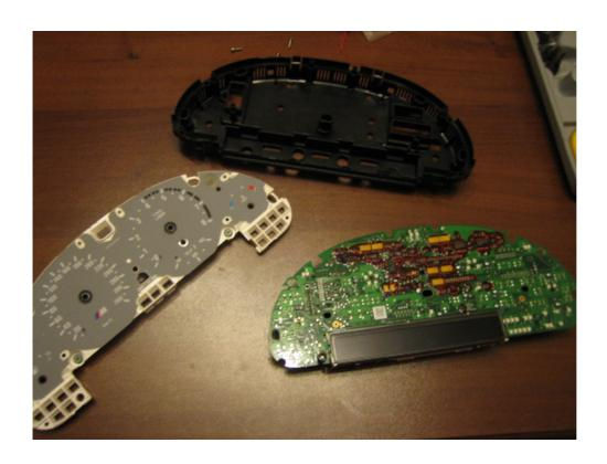
If you made it this far you have paid close attention. You will realize that the Pixel Display cover is attached to the board with screws and with four pins that are clipped around the base of the Display. These can be removed by applying pressure to disengage the clip. It may be necessary to use a pliers to reinstall. Apply pressure to get them to reconnect watching carefully not to cause damage.
