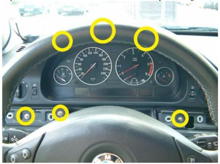
Once the screws have been removed, the frame can be tilted toward you (arrow direction) to remove it.
