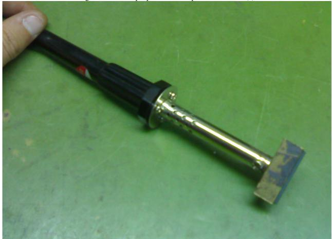
Once here, use a soldering iron with the proper head to repair the filament(s)
