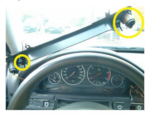
This picture shows the cluster being removed with the screw locations circled.
