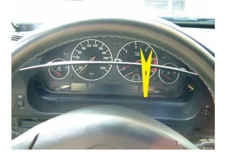
This picture shows the frame removed with two of the screw locations circled.
