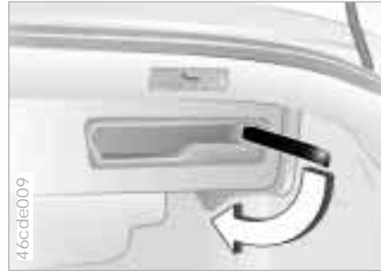
Lashing eyes are located on the inside corners of the luggage compartment for attaching luggage nets\* or elastic straps so that you can secure your luggage.
