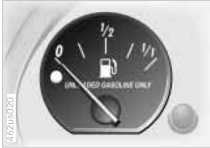
When you switch on the ignition, the indicator lamp lights up briefly as an operation check.
