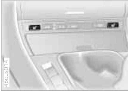
The seat cushion and backrest can be heated when the ignition key is in position 2.
