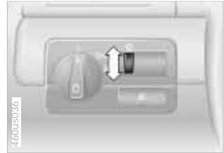
Turn the rotary dial to adjust the illumination intensity.
