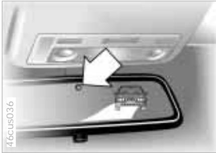
The semisolid reacts chemically to this electrical current, dimming the mirror through an infinitely-variable range (electrochromic technology).
