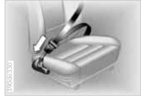
The safety belt tensioners respond to severe head-on collisions by tightening the belts to ensure that occupants remain firmly positioned in their seats. A gas-pressure system retracts the buckle assembly to tension the shoulder and lap belts within fractions of a second. This reduces the tendency to slide under the lap belt.
