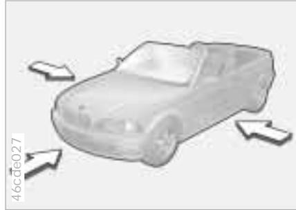
The illustration depicts schematically the primary directions of vehicle impact that initiate airbag deployment.
