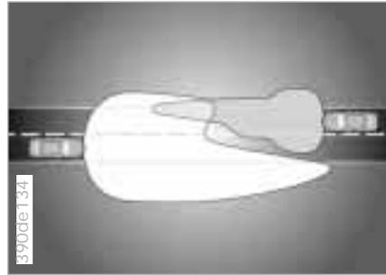
Xenon lamps illuminate the side and front areas of the vehicle with significantly more brightness and uniformity than the traditional halogen lamp.
