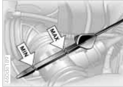
When the oil is between the two marks on the dipstick, there is approx. 1.1 US quarts (1 liter). Do not fill beyond the upper mark on the dipstick. Excess oil will damage the engine.
