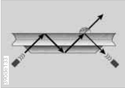
When the system is set to the "Intermittent" wiper speed, the wipers react immediately – if water is splashed onto the windshield by vehicles traveling ahead of you, for example. As a result, the rain sensor contributes to driving safety and comfort.
