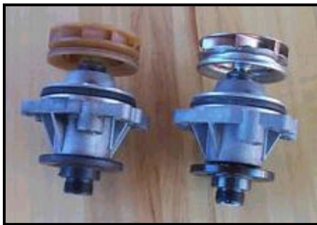
Water Pumps: Plastic Impeller (left) and Metal Impeller (right) (image courtesy of Ben Liaw)
